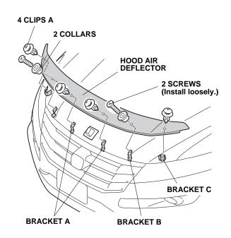
12. Insert the large end of the template between the hood and the hood air deflector to unfold the molding as shown. Remove the template by pulling it towards you.
